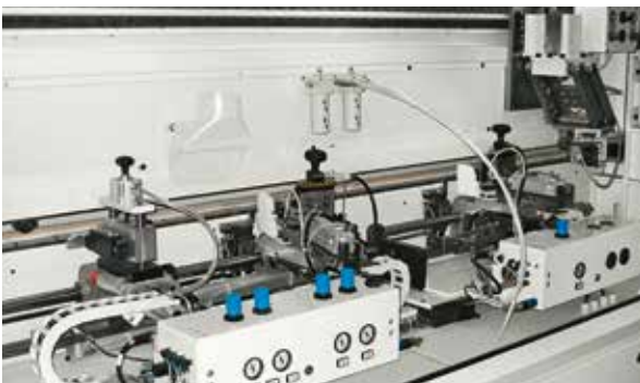
Corner finishing units for doors edgebanded on 3 or 4 sides.
