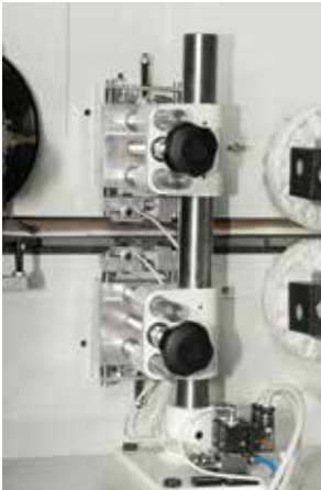
For the removal of any residual glue from the surface of the panel.
