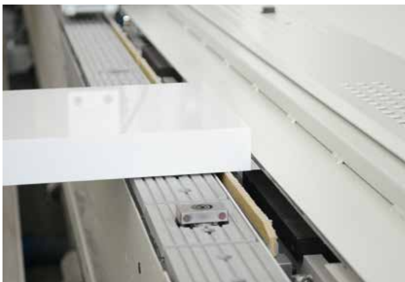
Lifting and waiting system of dogs with more sectors that allow to maximize productivity with each panel size.
