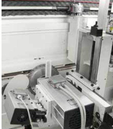
Hogging + scoring unit. Ideal for veneer panels.
