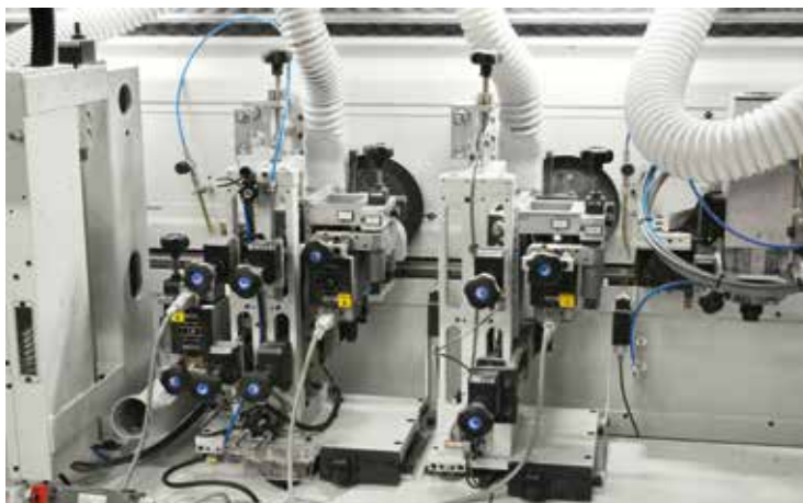
Shaping unit for the preparation of the coplanar joint, top or top+bottom, and for the realization of small radii up to 12 mm.
