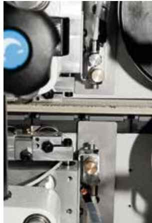
Spray device for the lubrication of the blades and for the brightening of ABS edges.
