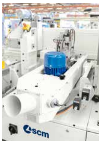
Sanding units for the finishing of doors machined with veneer edge.
