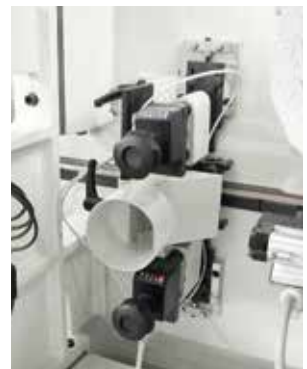
Scraping unit for the removal of the excess edge and the finishing of the profile.
