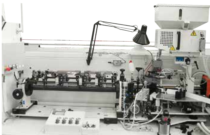
Gluing unit for the processing of doors with thin/soft edges.
