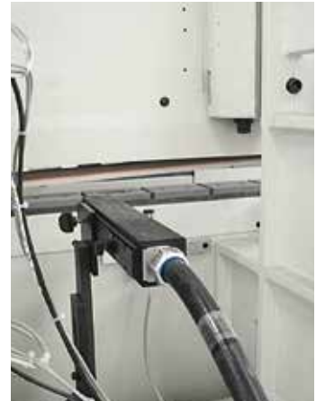
Inkjet printer for the marking of the panel in the upper or lateral surface.
