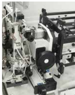
Longitudinal shear unit for the engraving of the excess edge.
