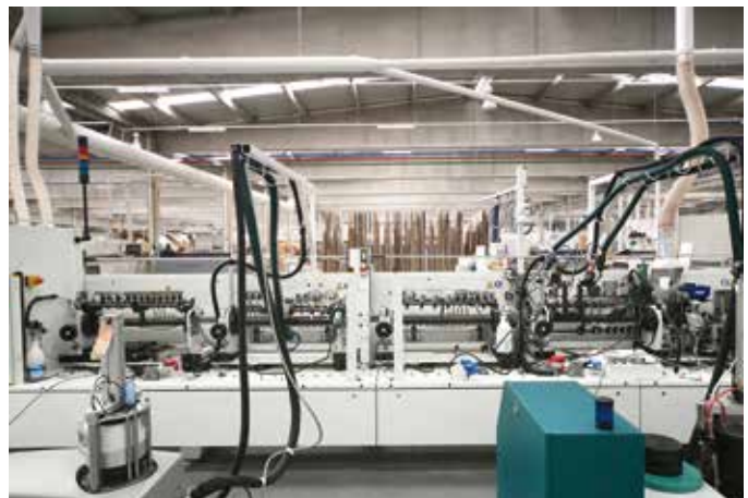
Gluing unit for softforming with pressure zone up to 4.5 m long. Ideal for any type of profiles with edge thicker than 0.8 mm and EVA/PU glue.
